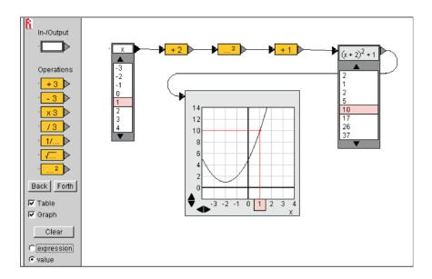
This program provides an interactive way of creating function machines with one instance of the variable. It allows learners to explore connections between the machines, algebraic formulae, tables of numbers and graphs.
